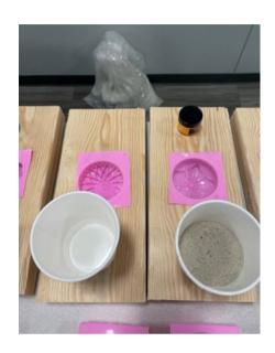
The quickset cement and the water must be stirred in the bowl and stirred in less than 5 minutes to avoid initial hardening:
