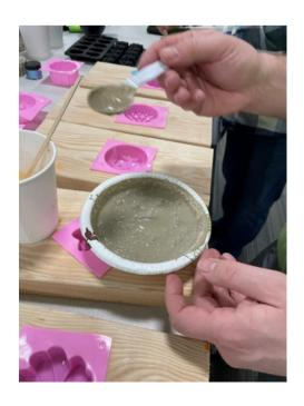
After stirring, the newly mixed concrete must be carefully poured into the silicone mold in layers or spooned into the mold in layers:
