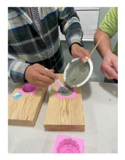
After each layer of concrete is spooned into the mold, the wooden form needs to be shaken by hand to get the internal bubbles in the wet concrete out. You should be able to see the bubbles burst on the surface of the concrete, if no more bubbles come out you can continue with the next layer or next step. In the photo below you will see they are using a concrete vibrator to remove the bubbles. You will be done by hand by tapping and vibrating the wood mold until bubbles in the concrete are
