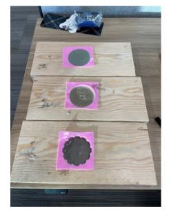
The dried pieces can be unmolded by lifting the silicone from the newly set concrete. Notice in the pictures that in some cases the bubbles were not totally removed, and cavities were created on the surface.
